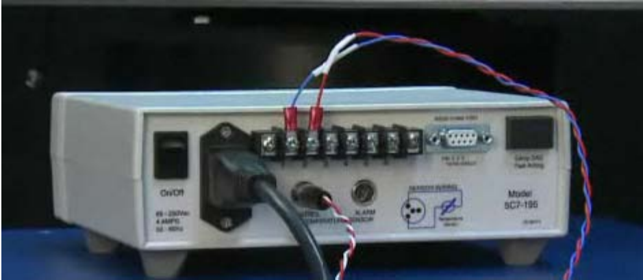
Figure 4-15. TEC Connection if equipped with external controller i
